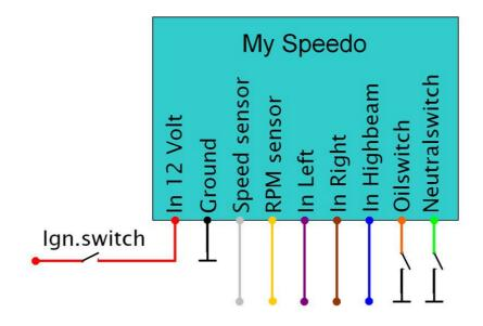
The connections are indicated like in the range of the original board.
